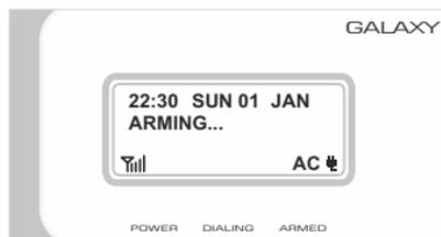
Delay arming beeps will sound from the remote keypad during the exit delay.
